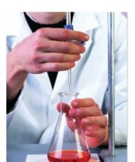
Figure 1 This acid-base titration is using methyl orange as an indicator. Methyl orange is coloured red in acidic solutions and yellow in basic solutions. The end point is the colour in between - orange. The solution in the conical flask above has reached the end point.
