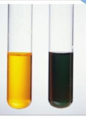
Figure 3 Oxidation of propan-1-ol to propanal with acidified potassium dichromate (VI) involves a colour change.
