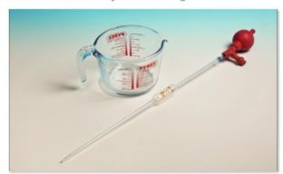
**Figure 4** A bulb pipette has less resolution than a measuring jug but is more accurate at measuring 25 cm<sup>3</sup> of liquid at 25 °C.
