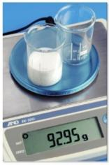
**Figure 1** A top pan balance has an accuracy of  $+/-0.01\,\mathrm{g}$ , so the mass should be reported to two decimal places.
