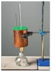
**Figure 2** Using copper calorimetry. Find out more about copper calorimetry in topic 3.2.5.
