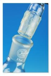
Figure 2 Quickfit joints must be secured.
