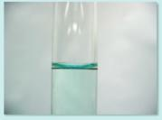
Figure 1 A volumetric flask. Figure 2 The correct position of the meniscus.
