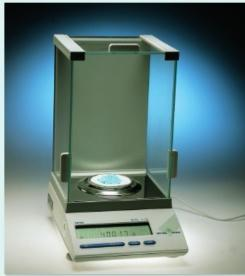
**Figure 2** An analytical mass balance, which allows the mass of substances to be determined to a high degree of accuracy.
