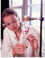
**Figure 2** A chemist using a separating funnel in an organic synthesis. Find out more about organic techniques in topic 4.2.7.
