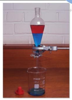
**Figure 5** A separating funnel can be used to separate immiscible liquids.
