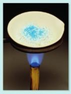
Figure 2 Heating hydrated copper sulfate. Although this experimental method is easy to carry out, it will only work if the anhydrous salt is not decomposed by heat. Unfortunately, many salts are decomposed by heat. This is especially true for nitrates.
